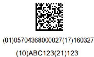
Figure 14: Example of GS1 DataMatrix containing GTIN, Expiration date, Batch/Lot number and Serial number
