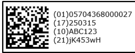
Figure 14: Example of GS1 DataMatrix containing GTIN, Expiration date, Batch/Lot number and Serial number
