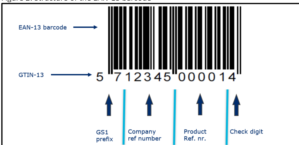
Figure 2: Structure of the EAN-13 barcode
